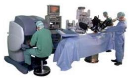
The Surgical Cart that includes the **EndoWrist** Instruments. The **EndoWrist** Instruments are designed to mimic the movement of the human hands, wrists and fingers.
